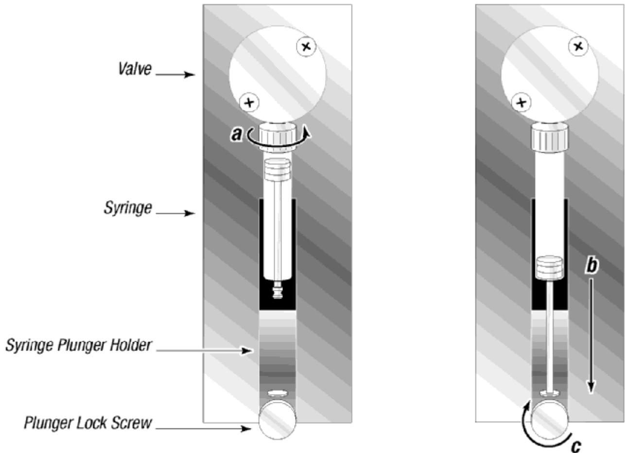
**Figure 2-11. Syringe Installation**
