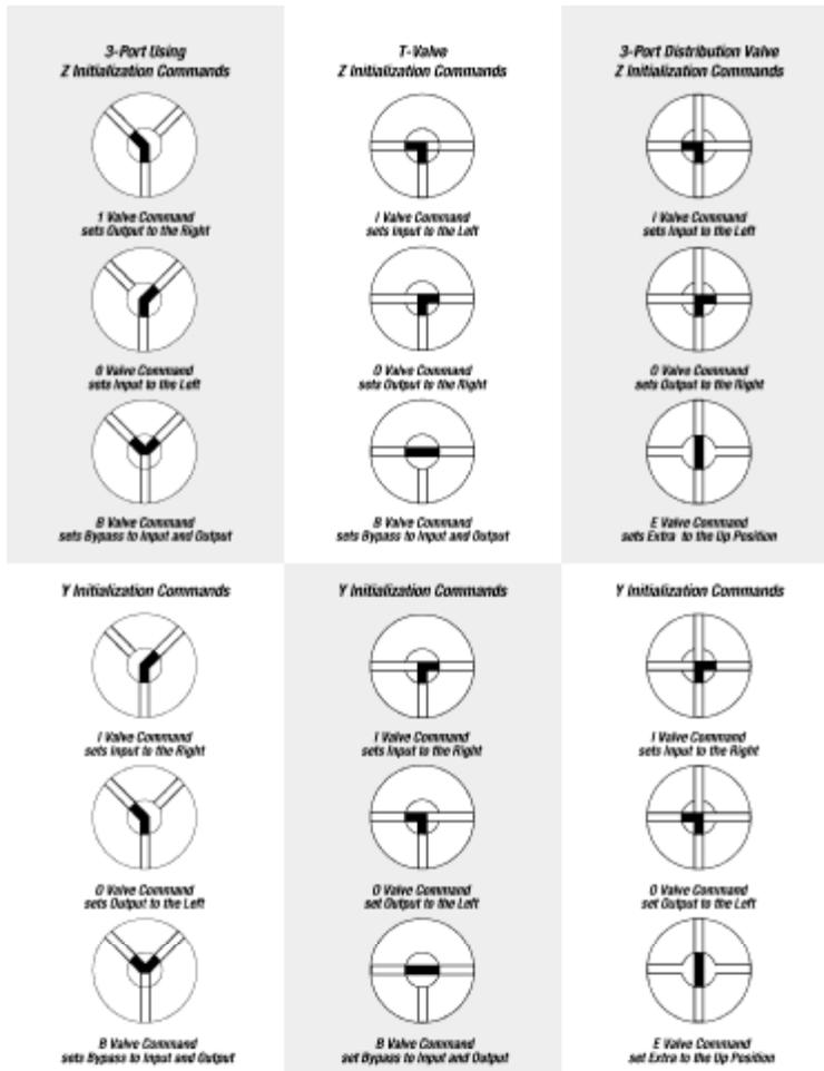
Figure 3-1. Valve Positions for all Valve Types
