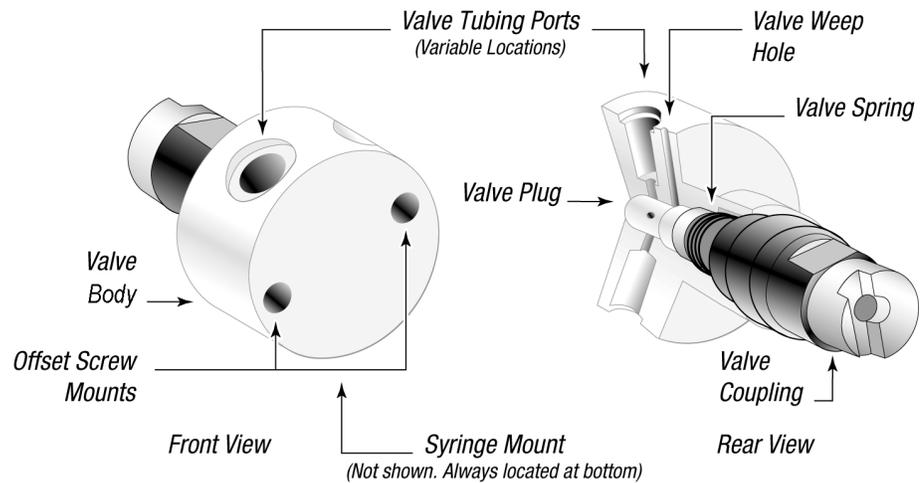
**Figure 2-10. XP 3000 Valve Installation (3-Port Valve Shown)**
