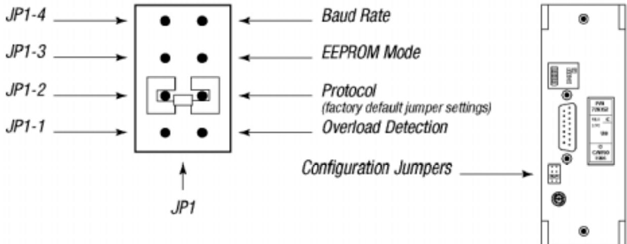
Figure 2-6. Configuration Jumpers
