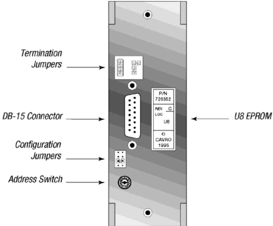
**Figure 1-4. XP 3000 Printed Circuit Board External Connectors**
