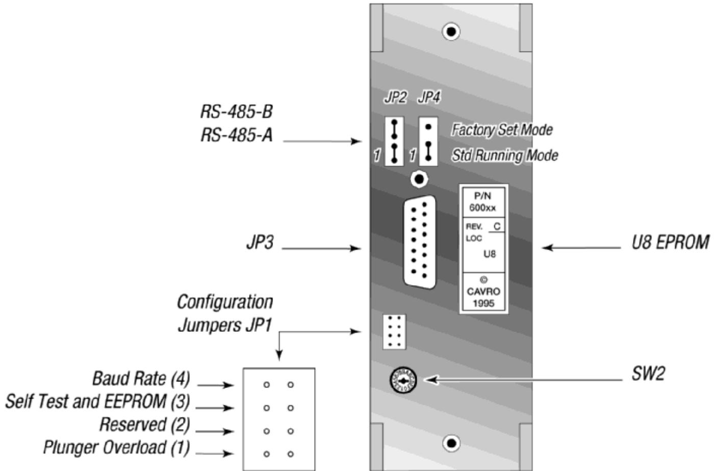
Figure 2-8. Printed Circuit Board Settings for Microstep-Enabled Firmware
