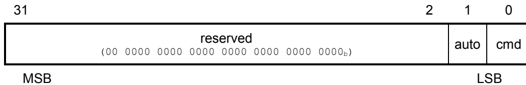
Figure 56: Storage read access structure
