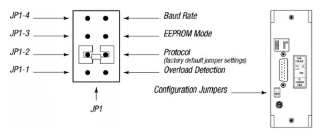
Figure 2-6. Configuration Jumpers
