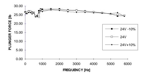
Figure B-1. Plunger Force Curve
