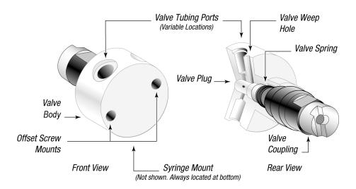
Figure 1-3. 3-Port Valve Components
