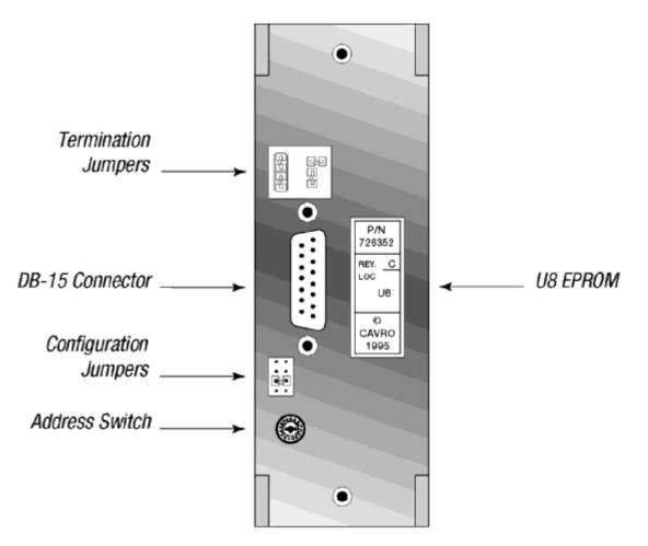
Figure 1-4. XP 3000 Printed Circuit Board External Connectors
