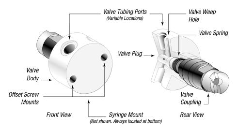
Figure 5-3. XP 3000 Valve Replacement (3-Port Valve Shown)
