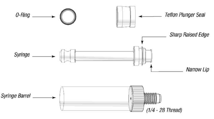
Figure 1-2. Syringe Components
