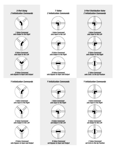
Figure 3-1. Valve Positions for all Valve Types
