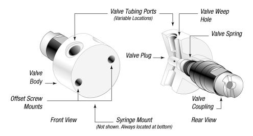
Figure 2-10. XP 3000 Valve Installation (3-Port Valve Shown)
