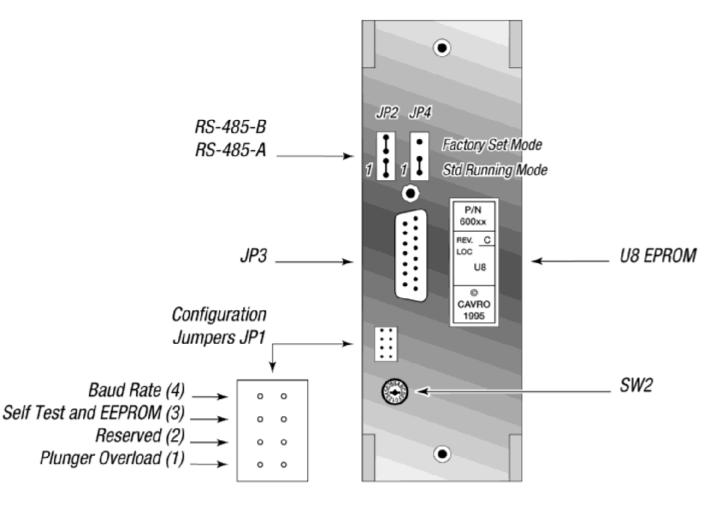
Figure 2-8 shows the printed circuit board settings for the microstep-enabled firmware.
