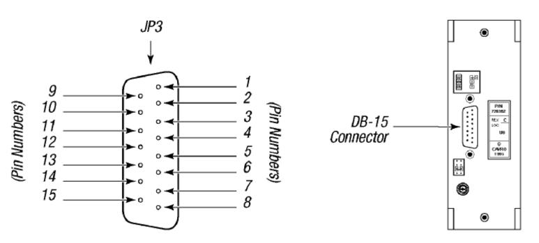
Figure 2-1. DB-15 Connector Pins
