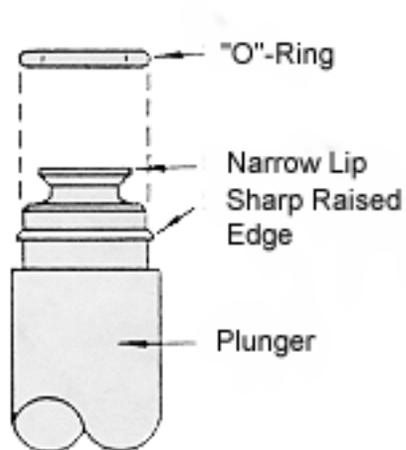
**Caution:** 5.0 mL, 10.0 mL and 25.0 mL syringes have "O"-rings beneath the seal. Be careful not to damage the "O"-ring. If it is necessary to replace the "O"-ring, simply slip the new "O"-ring over the narrow lip on the plunger. It may be necessary to use needle nose pliers to assist in removing the "O"-ring from the 10.0 mL and 25.0 mL plunger.
