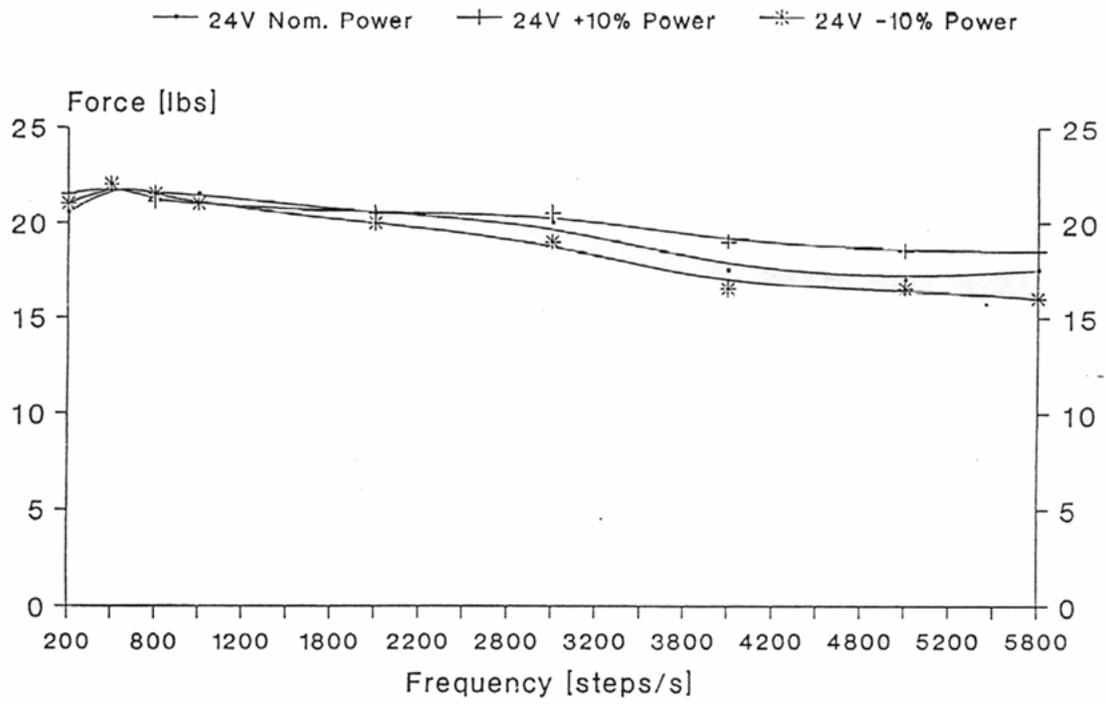
**Figure 10. XL 3000 High Resolution Pump Typical Plunger Force Curve (Dynamic Force)**
