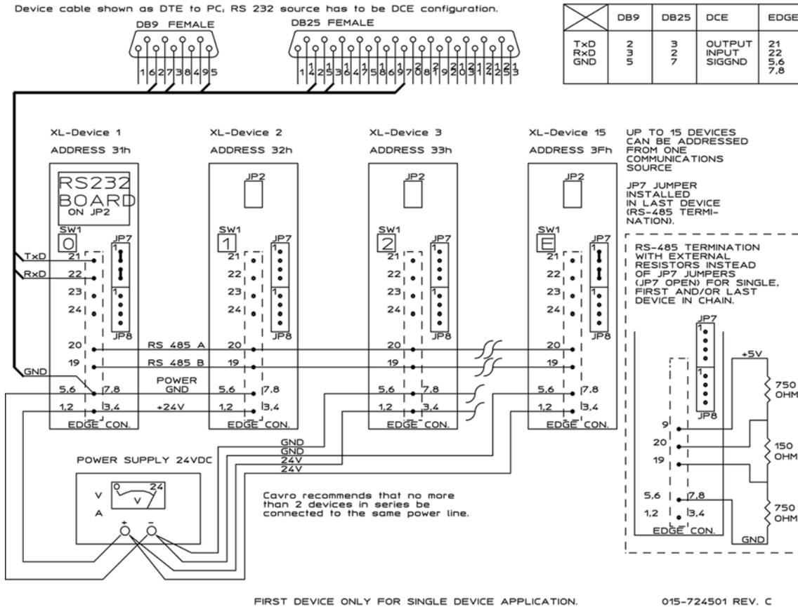
**Figure 4. Cabling Illustration: RS-485 Multipump Cabling**
